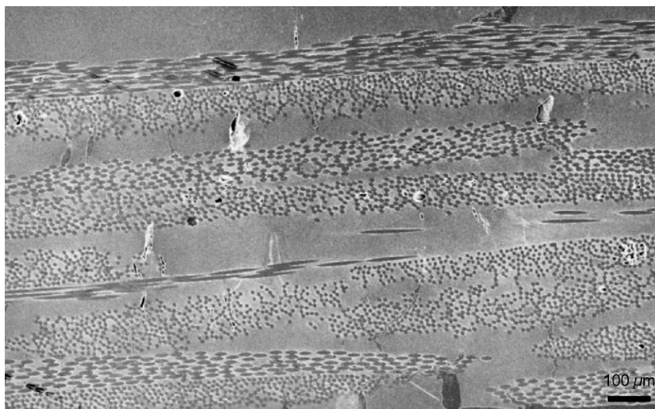
Fig. 9. SEM micrograph of a Nextel™ 720 fibre-reinforced alumina matrix composite containing four fibre layers (fibre mats) fabricated by simultaneous electrophoretic deposition. The sample was sintered at 1300^\circ\text{C} for 1 h.
